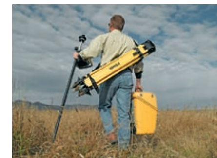
Topographic surveying – in Robotic mode one person can measure and log points as fast as he or she can walk.
