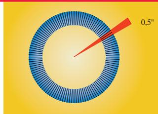
The total stations have a specially-manufactured angle measuring system that facilitates a measuring accuracy of 0.15mgon (0.5") on the TC2003 and TCA2003. Key elements here are the precise drives and the quadruple detection of the graduated circles.
