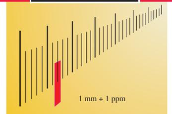
All total stations are equipped with coaxial precision distancers. On the TC2003 and TCA2003, a distance measuring accuracy of 1mm +1ppm is achieved due to the use of specially-developed components.
